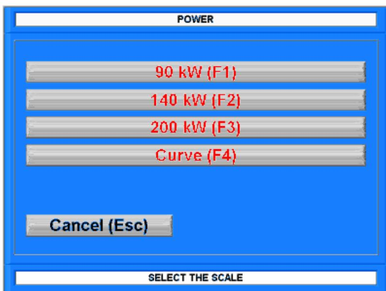
After selecting the presumed power, the page with the diagram and the message "Press the clutch before exceeding the rpm" appears at the bottom of the screen.
